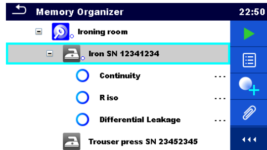
Figure 5.3: Example of status - No measurement result(s)
