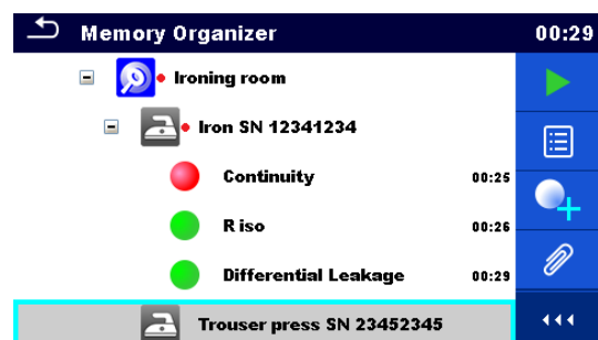
Figure 5.5: Status - Measurements completed with fail result(s)
