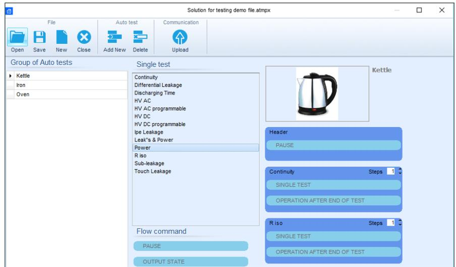
User defined structure with measurements and limits can be created on the PC SW and then uploaded to instrument.
