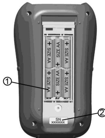
Figure 3.4: Battery compartment
