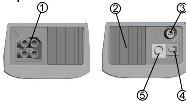
Figure 3.2: Connector panel
