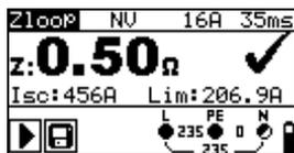
Figure 5.25: Example of loop impedance measurement result
