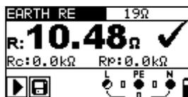
Figure 5.35: Example of earth resistance measurement result
