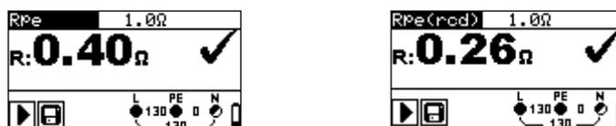
Figure 5.40: Examples of PE conductor resistance measurement result
