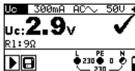
Figure 5.18: Example of contact voltage measurement results
