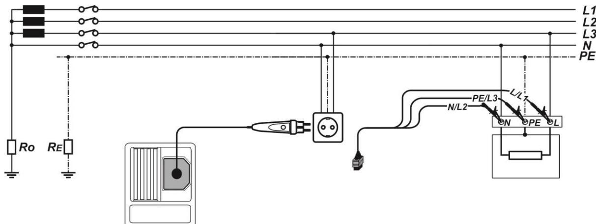
Figure 5.24: Connection of plug commander and 3-wire test lead
