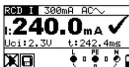
Figure 5.20: Trip-out current measurement result example
