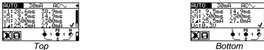
Figure 5.22: Two parts of result field in RCD auto-test
