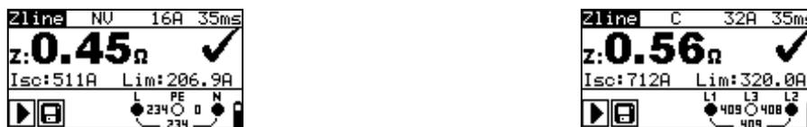
Figure 5.29: Examples of line impedance measurement result
