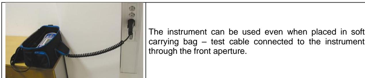
The instrument can be used even when placed in soft carrying bag – test cable connected to the instrument through the front aperture.
