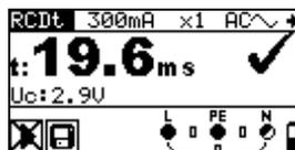
Figure 5.19: Example of trip-out time measurement results
