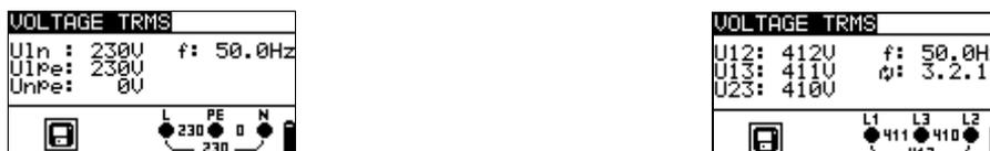
Figure 5.4: Examples of voltage measurement in three-phase system
