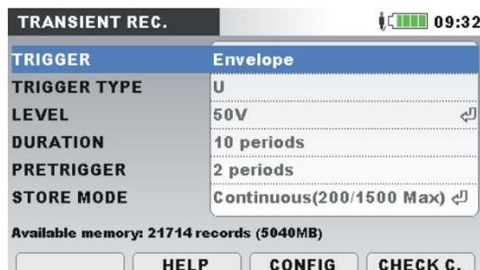
Figure 95: Transient setup screen – MI 2892/MI 2885
