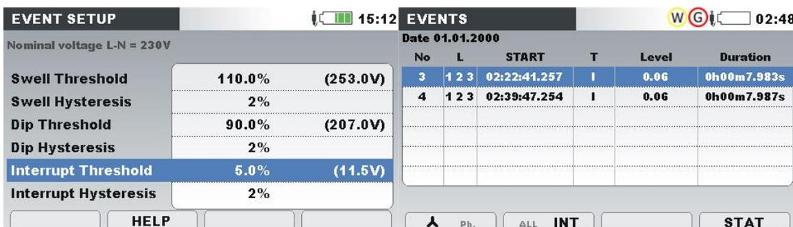
Figure 163: Voltage interrupts related screens on the instrument
