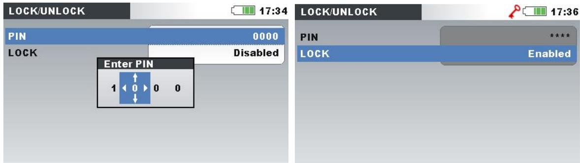
Figure 102: Lock/Unlock screen
