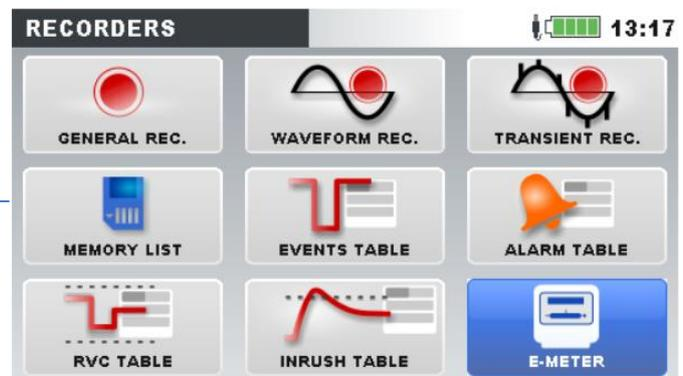
Figure 14: Recorders submenu (MI 2892/MI 2885)
