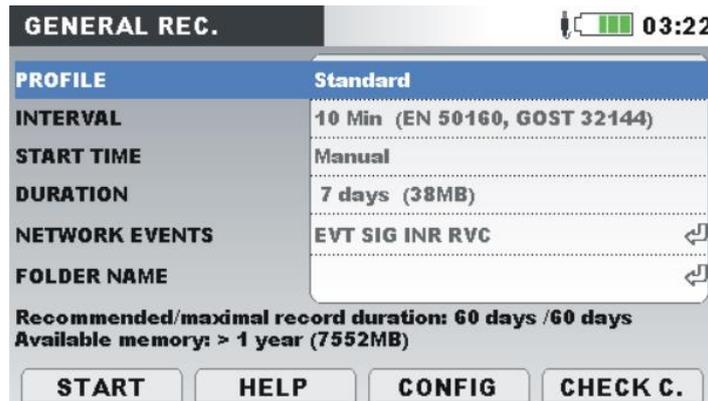
Figure 56: General recorder setup screen
