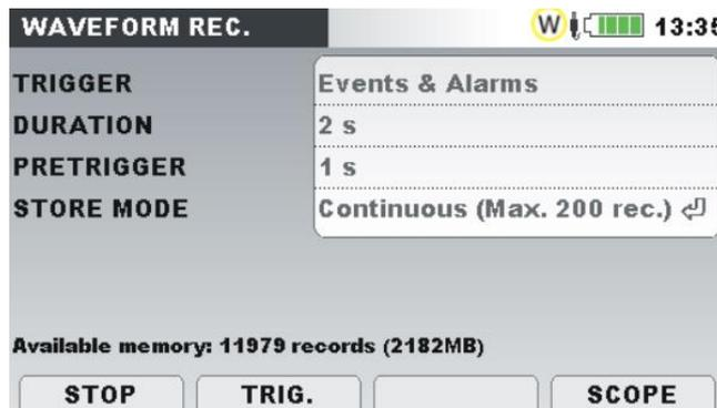
Figure 60: Waveform recorder screen
