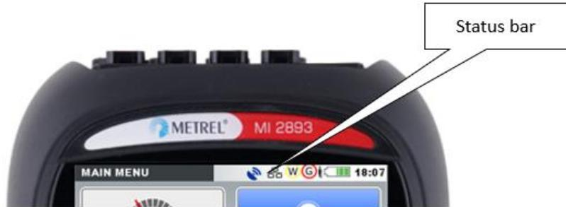
Figure 9: Instrument status bar
