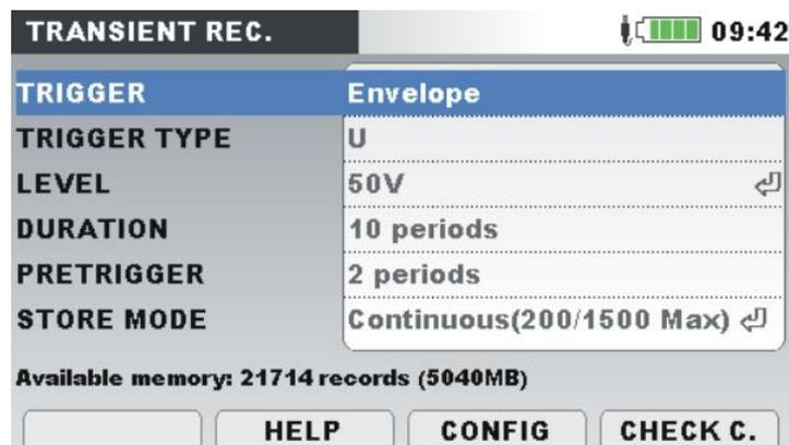
Figure 64: Transient recorder setup screen – MI 2892/MI 2885
