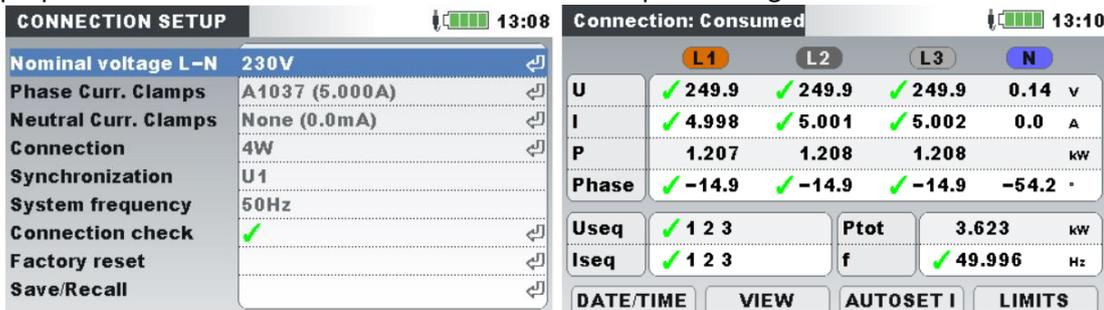
Figure 76: PQA setup connection and Connection check
