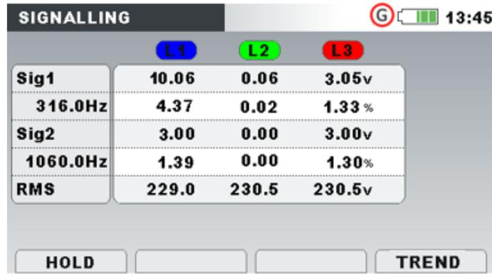
Figure 53: Signalling meter screen
