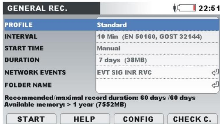
Figure 179: Predefined EN50160 recorder configuration
