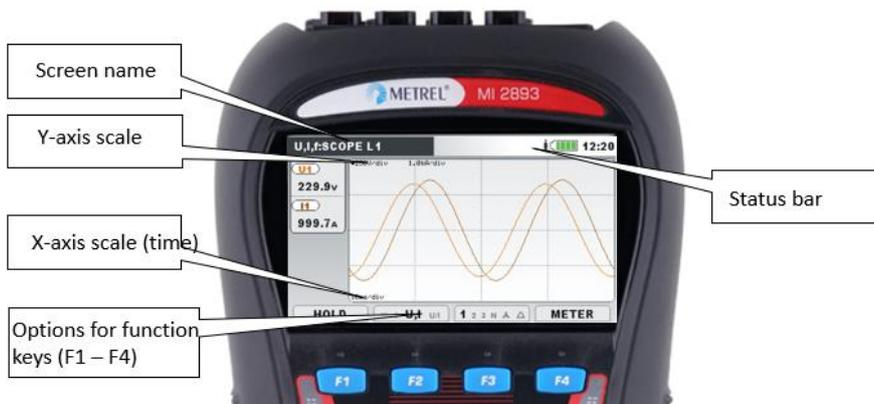
Figure 8: Common display symbols and labels during measurement campaign
