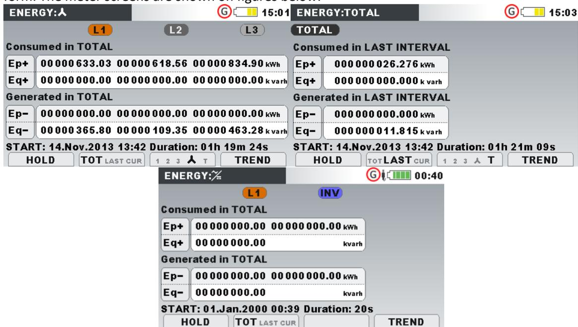
Figure 35: Energy counters screen (General Recorder is running)
