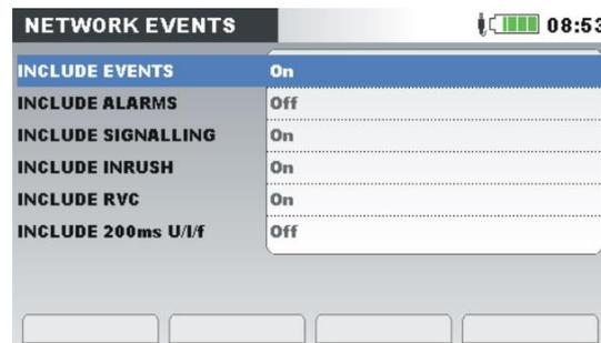
**Note:** Waveform duration and pretrigger for event and alarms captured under General Recorder are programmed under [EVENT SETUP](#) and [ALARM SETUP](#) window.
