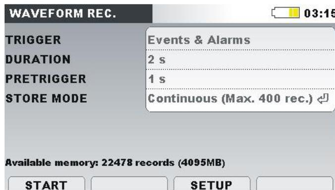
Figure 59: Waveform recorder capture screen
