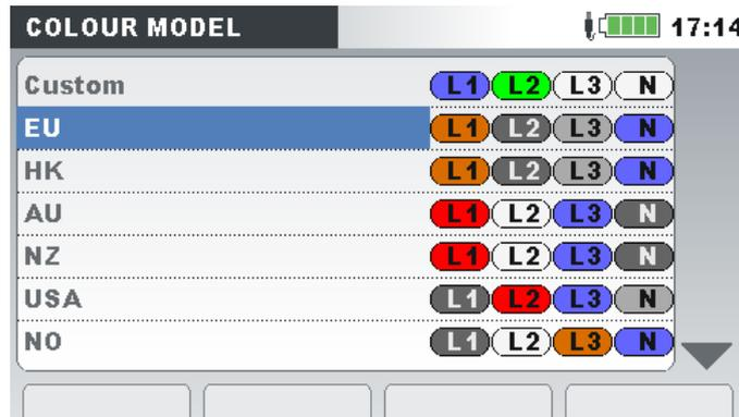
Figure 104: Colour representation of phase voltages
