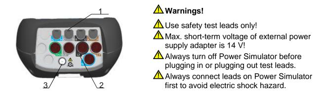
Figure 2.2: Front connector panel
