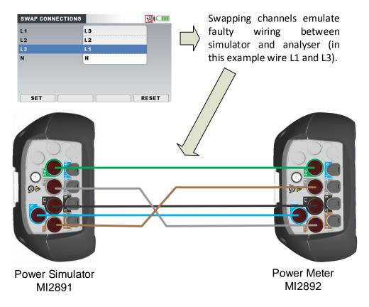
Figure 3.8: Swapping instrument channels
