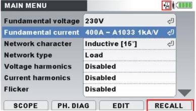
Figure 62: RECALL function key
