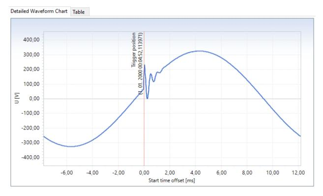
Figure 3.37: Generated transient sample, captured by MI 2892 Power Master
