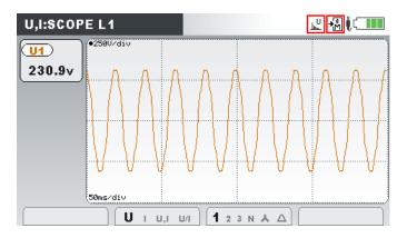
Figure 3.15: 230V fundamental voltage signal with added 5% of 3<sup>rd</sup>, 5<sup>th</sup> and 7<sup>th</sup> harmonic
