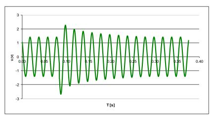
Figure 3.32: Inrush on voltage
