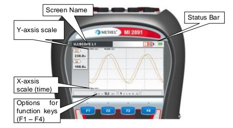
Figure 3.2: Common display symbols and labels on SCOPE screen
