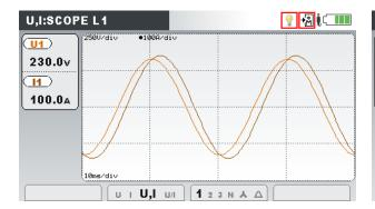
Figure 3.11: Voltage and current waveform (single mode)
