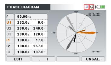
Figure 3.13: Phase diagram screen
