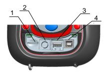
Figure 2.3: Upper connector panel
