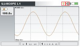
Figure 3.10: Current only waveform
