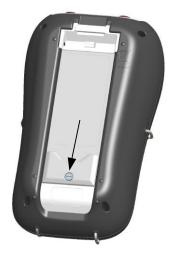
Figure 7.2: Closing the battery compartment cover
