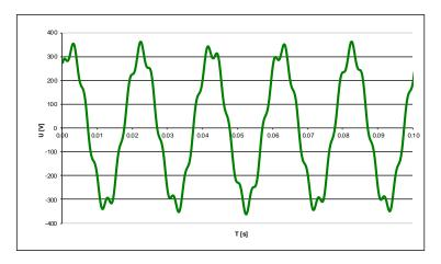
Figure 3.35: Generated signalling, 10 % U<sub>Nom</sub>, signalling frequency 316.0 Hz
