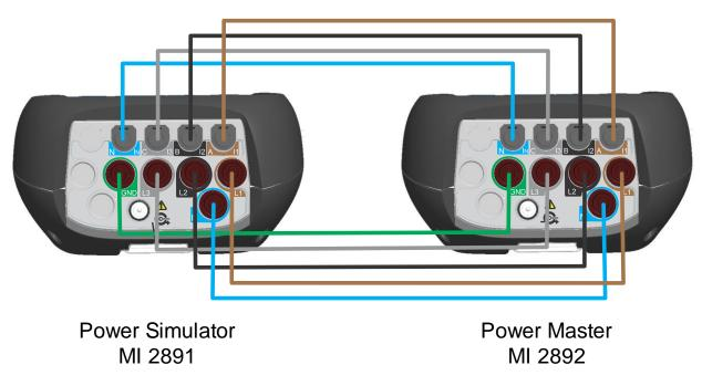
Figure 5.1: Recommended lead connection
