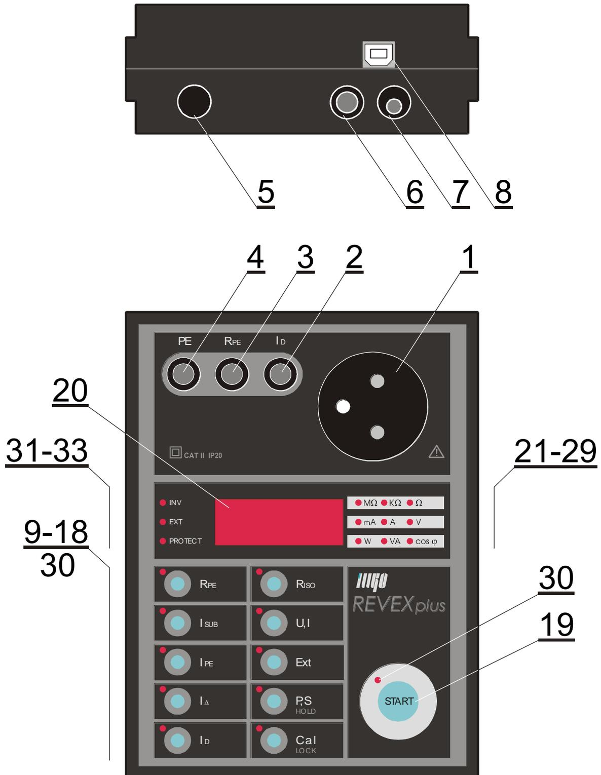
Fig. 1 – Front panel and rear panel
