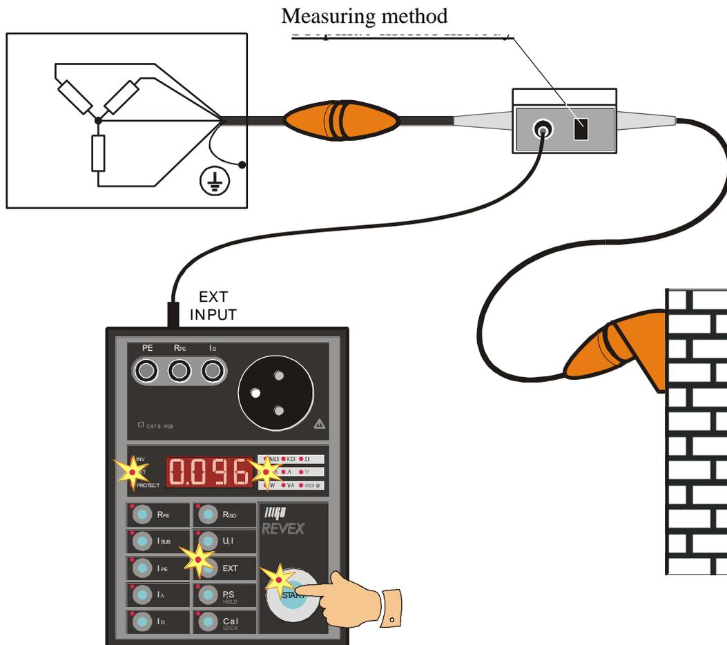
Fig. 9 – Three-phase adapter connection
