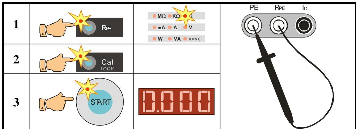
Fig. 3 – Test lead resistance compensation
