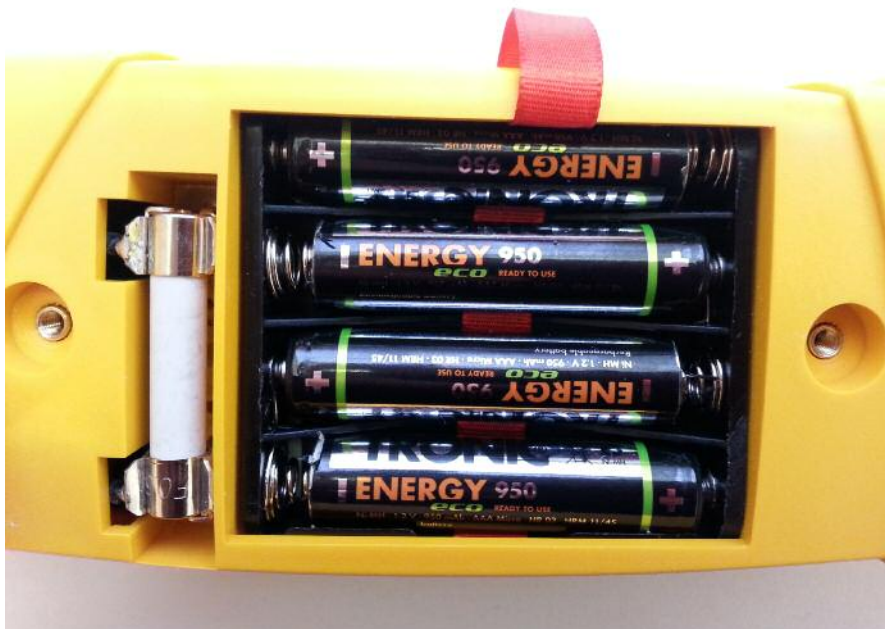
Fig. 4.1 Correct batteries / accumulators polarity and the fuse location
