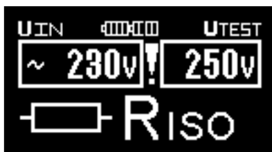
Fig. 3.4a Example of voltage measurement (RISO function)
