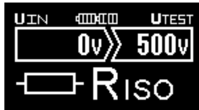
Fig. 3.5 Example of setting for insulation resistance measurement
