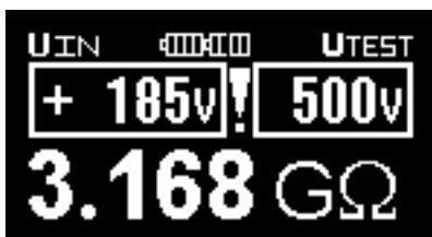
Fig. 3.7a Example of RISO measurement result (discharging in progress)
