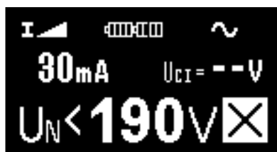
Fig. 3.14 Example of settings for trip-out current measurement
