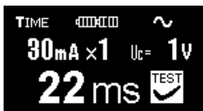
Fig. 3.12a Example of trip-out time measurement result
