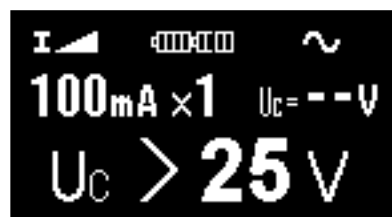
Fig. 3.4b Contact voltage > 25 V
