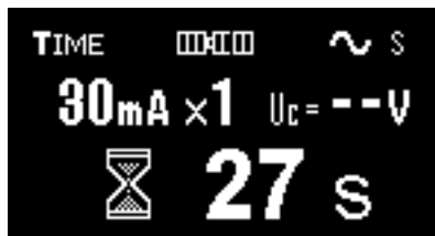
Fig. 3.13 Example of count down for selective RCD
