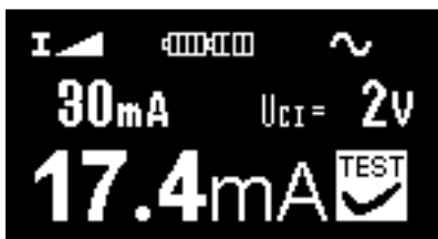
Fig. 3.15a Example of trip-out current measurement result
