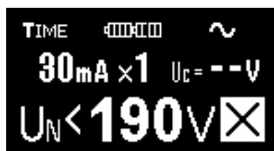
Fig. 3.11 Example of settings for trip-out time measurement
