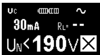
Fig. 3.8 Example of settings for contact voltage measurement
