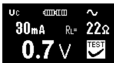
Fig. 3.10 Example of contact voltage measurement result
